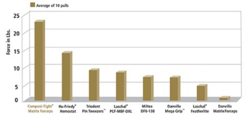
Testing was performed using a pull force gauge with .0013" matrix material. Each forceps was tested for 10 pulls, with the average force shown in the chart below.
